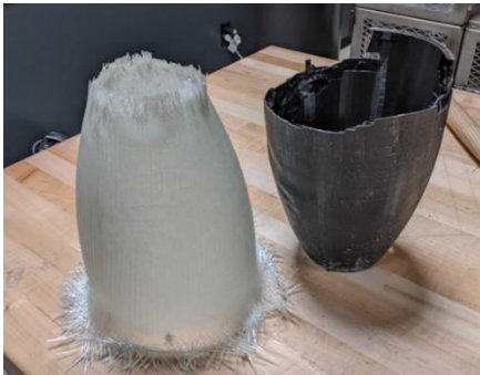
Fig.4 Tailcone mold for fiberglass lay up
