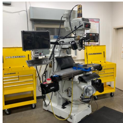
Fig. 1 Manual mill with a computer used by students completing the formal mill and lathe training
